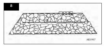
• Lean the granite chippings against the burner ledges to disguise the ledges, Diagram 9
